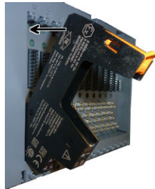
Figure 2-5: CHARM Terminal Block installation
