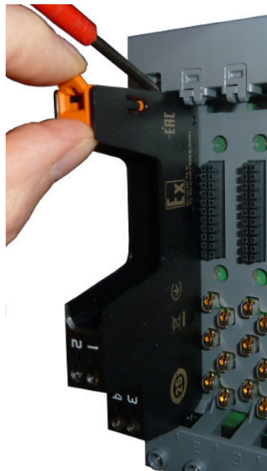
Figure 6-2: Remove a Terminal Block
